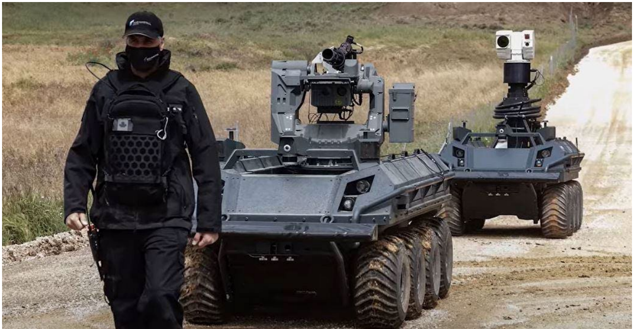
Mission Master SP's modular design: same platform with different payloads
